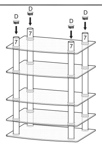
Insert caps (D) into cylinders (7). Note that caps (D) may come pre-inserted into cylinders (7).
